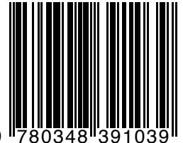
A standard EAN-13 barcode representing the ISBN 978-0-348-39103-9. It consists of vertical black bars of varying widths on a white background.
