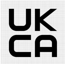
2. Where the UK marking is reduced or enlarged, the proportions given in the graduated drawing in paragraph 1 must be respected.
