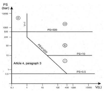
(d) (i) Table 4: Vessels for liquids having a vapour pressure at the maximum allowable temperature of not more than 0.5 bar above normal atmospheric pressure (1013 mbar) and, for fluids in Group 2 with a pressure PS greater than 10 bar and a product of PS and V greater than 10000 bar.L, or with a pressure PS greater than 1000 bar
