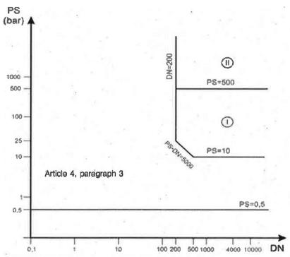
(i) Table 9: Piping intended for liquids having a vapour pressure at the maximum allowable temperature of not more than 0.5 bar above normal atmospheric pressure (1013 mbar) and, for fluids in Group 2 with a PS greater than 10 bar, a DN greater than 200 and a product of PS and DN greater than 5000 bar
