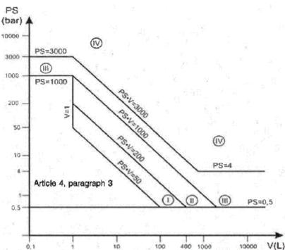
than 1L and a product of PS and V is greater than 50 bar.L, or a pressure PS greater than 1000bar  $\,$
