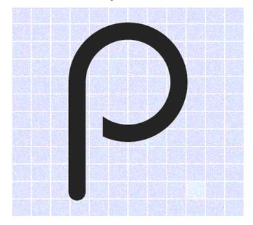
2. Where the marking is reduced or enlarged, the proportions given in the graduated drawing in paragraph 1 must be respected.
