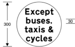
954.7 Same as diagram 954 applying to buses, taxis and pedal cycles where the signs are mounted in combination with light signals prescribed by regulation 33
