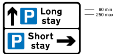
2505 Directions to different types of parking place from a junction ahead
