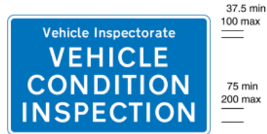
832.2A Vehicle condition check point ahead
