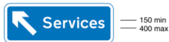
2921.1 Same as diagram 2921 or direction to a motorway service area at a junction ahead on a motorway slip road
