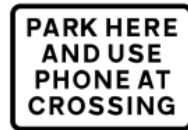
786 Place where large or slow, or long low vehicles should wait near a railway or tramway level crossing while the driver obtains permission by telephone to cross or confirms he has crossed
