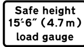
780.2A Safe height beneath electrified overhead cable ahead provided with a load gauge shown in diagram 781
