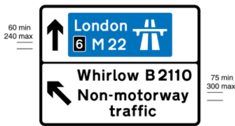
2124.1 Junction ahead of a non-primary route which leads directly onto a motorway, with another non-primary route which should be followed by traffic not wishing or permitted to use the motorway
