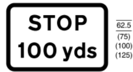
502 Distance to a junction ahead controlled by a diagram 601.1 ("STOP") sign
