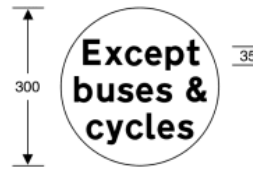
954.6 Same as diagram 954 applying to buses and pedal cycles where the signs are mounted in combination with light signals prescribed by regulation 33
