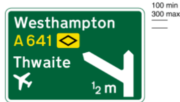
2011 Grade separated junction 1/2 mile ahead of a primary route with another primary route which leads to an airport and which forms part of an emergency diversion route
