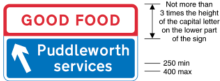
2920.1 Direction to a named motorway service area and showing the name of the operator
