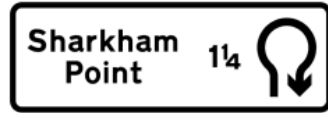
2111.1 Direction along a non-primary route to a destination shown via a U-turn at a roundabout ahead
