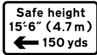
780.1A Safe height beneath electrified overhead cable in direction and at distance indicated
