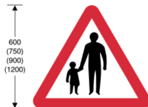
544.1 Pedestrians in road ahead
