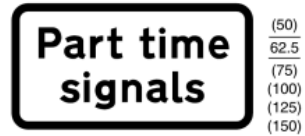
543.1 Traffic signals ahead which only operate at certain times
