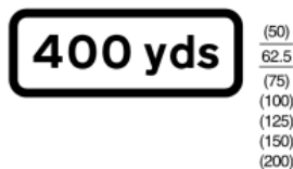
572 Distance ahead to hazard
