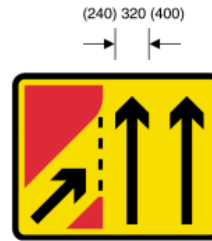
7252 Traffic joining from the left at a junction as part of temporary traffic management scheme; traffic on the main carriageway has priority
