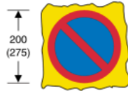
636 Temporary prohibition of waiting except for loading and unloading
