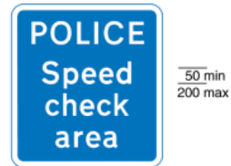
829.5 Area where police carry out checks on the speed of vehicles
