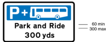
2503 Distance to a parking place ahead from which a 'Park and Ride' scheme operates
