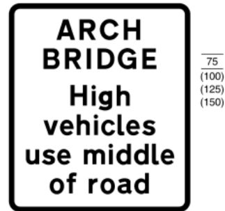
531.2 High vehicles to use the middle of road at arch bridge ahead
