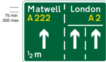
2017 Grade separated junction 1/2 mile ahead where the left hand lane of a primary route leaves the main carriageway of that route and leads to another primary route
