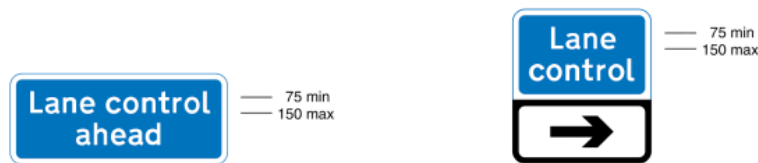
5012 System of lane control light signals ahead
