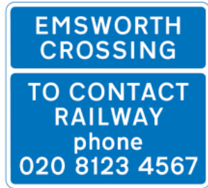
785.1 Name of level crossing and details of telephone number for contacting railway or tramway operator
