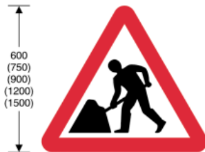
7001 Road works or temporary obstruction of the carriageway ahead
