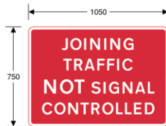
7022 Traffic joining a length of road being controlled by portable light signals is not controlled by such signals
