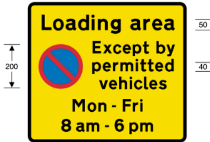
640.3 Entrance to a designated off-highway loading area in which waiting restrictions apply
