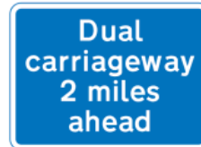
818.1 Distance to a section of dual carriageway road ahead
