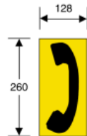
787 Site of emergency telephone or telephone at or near a railway or tramway level crossing
