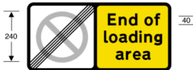
640.5 End of designated off-highway loading area in which waiting restrictions apply
