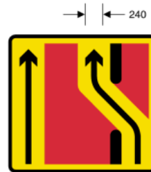
7216 Right hand lane returns to right hand side of original carriageway ahead, but remains separated by works area from left hand lane
