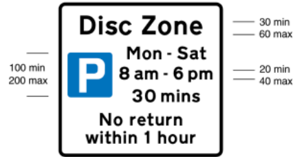
662 Period during which waiting is limited and display of a disc is required at a parking place in a disc zone
