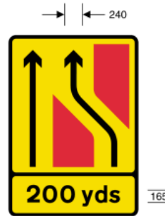
7239 Traffic diverted from right hand lane to rejoin centre lane
