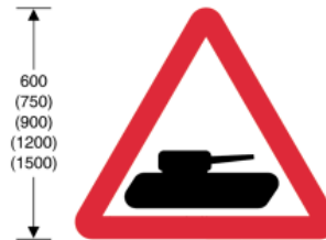
582 Slow moving military vehicles likely to be crossing or in road ahead
