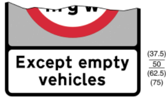
627.1 Exemption for unladen vehicles from the prohibition conveyed by the sign in diagram 626.2A
