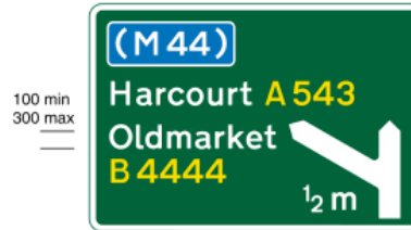
2012 Grade separated junction 1/2 mile ahead of a primary route with another primary route which leads to a motorway and with a non-primary route
