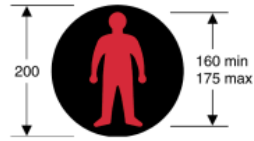
4006 Light signal at level crossing for pedestrians
