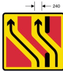
7217 Left hand lane returns from right hand side of original carriageway to left hand side ahead and right hand lane returns from other carriageway to right hand side of original carriageway
