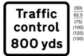
7030 Temporary traffic control ahead where vehicles are to be escorted in convoys through road works
