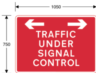
7021 Traffic on road ahead is being controlled by portable light signals (Indication to traffic joining that road)
