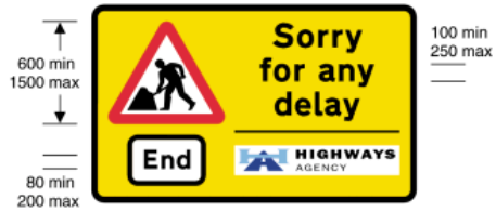
7006 End of road works and of any associated temporary statutory restrictions
