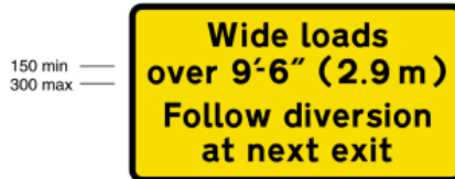
7292 Instructions to drivers of wide loads on action to be taken before reaching road works ahead
