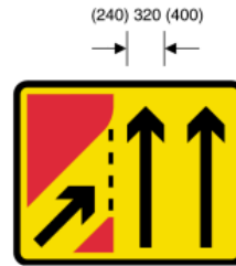
7252 Traffic joining from the left at a junction as part of temporary traffic management scheme; traffic on the main carriageway has priority
