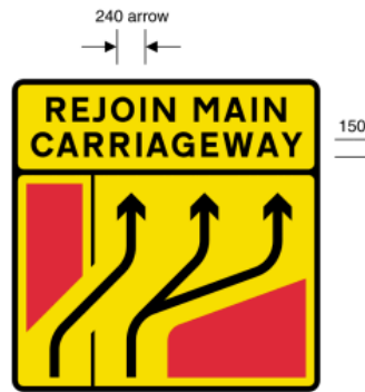
7232 Return of traffic from hard shoulder and left lane of carriageway to use three lanes
