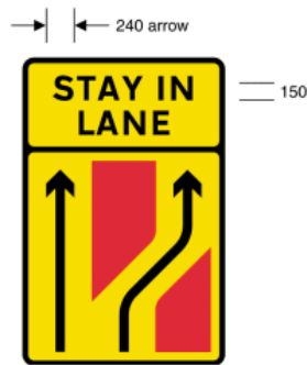
7238 Diversion of traffic from centre lane to right hand lane; traffic in left hand lane is unaffected
