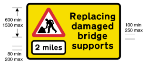
7004 Road works ahead and the nature of works indicated
