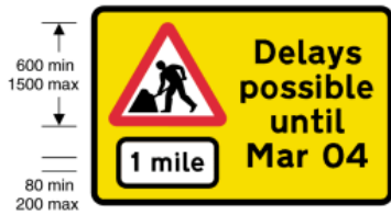
7005 Delays possible for specified period owing to road works ahead
