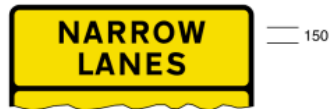
7264 Panel to appear at top of road works sign indicating that traffic lanes are narrower than normal
