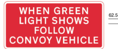
7028 Vehicular traffic must follow the vehicle escorting the convoy through the road works
