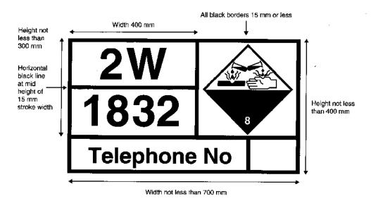
The emergency action code shall be inscribed in the upper half and the UN number in the lower half of the orange-coloured panel and the telephone number (or text as the case may be) beneath the UN number.
