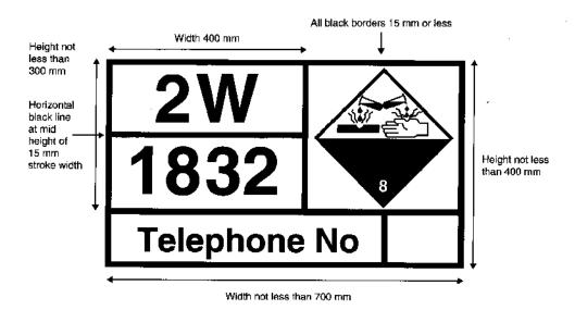
The emergency action code shalf be inscribed in the upper half and the UN number in the lower half of the orange-coloured panel and the telephone number (or text as the case may be) beneath the UN Number.
