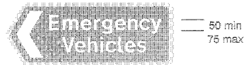
2710 Direction of route for emergency vehicles to an emergency services incident point
