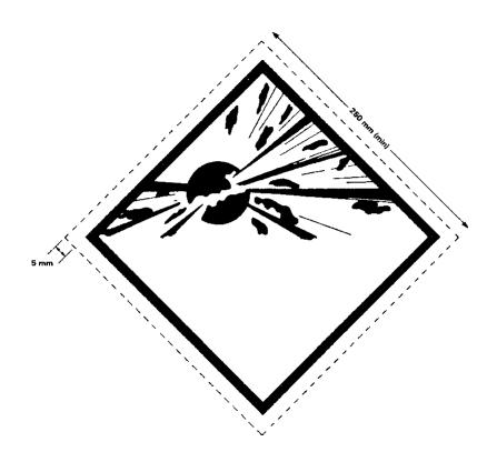
(b) comply with the measurements in the diagram, except that larger measurements may be used in which case the measurements shall be increased proportionally.
