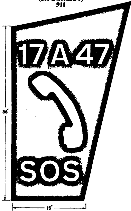
Side of emergency telephone box (See Direction 9) 914
