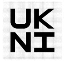
2. Where the UK(NI) indication is reduced or enlarged, the proportions given in the graduated drawing in paragraph 1 must be respected.
