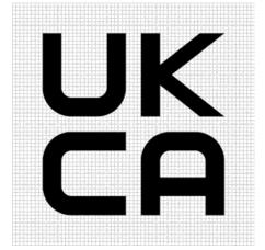
2. Where the UK marking is reduced or enlarged, the proportions given in the graduated drawing in paragraph 1 must be respected.
