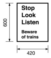
Upper section — White lettering on red backgroundLower section — Black lettering on white backgroundInstructions for use at a vehicular crossing without a telephone Diagram 102Permitted variant: Telephone number of crossing operator may be added.
