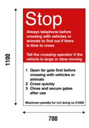
Upper section — White lettering on red backgroundLower section — Black lettering on white backgroundInstructions for use at a vehicular crossing with a telephone Diagram 103 Upper section — White lettering on red backgroundLower section — Black lettering on white backgroundInstructions for use at a vehicular crossing with a telephone Diagram 103
