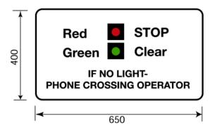
Black lettering and border on white backgroundSign for use with miniature stop lights at a crossing without a telephone Diagram 108Permitted variant: The lenses of the lamps may be rectangular instead of circular
