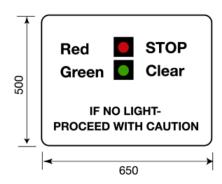
Black lettering and border on white backgroundInstructions for use at a crossing with miniature stop lights and user-operated gates Diagram 109
