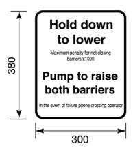
Black lettering and border on white backgroundSign indicating the penalty for failure to shut the gate at a vehicular crossing Diagram 105
