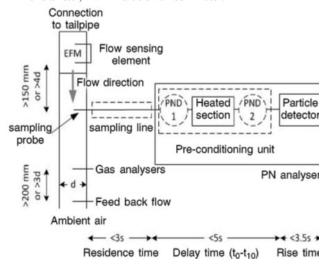
The PN analyser shall be connected to the sampling point via a sampling probe which extracts a sample from the centreline of the tailpipe tube. As specified in point 3.5 of Appendix 1, if particles are not diluted at the tailpipe, the sampling line shall be heated to a minimum temperature of 373 K (100 °C) until the point of first dilution of the PN analyser or the particle detector of the analyser. The residence time in the sampling line shall be less than 3 s.
