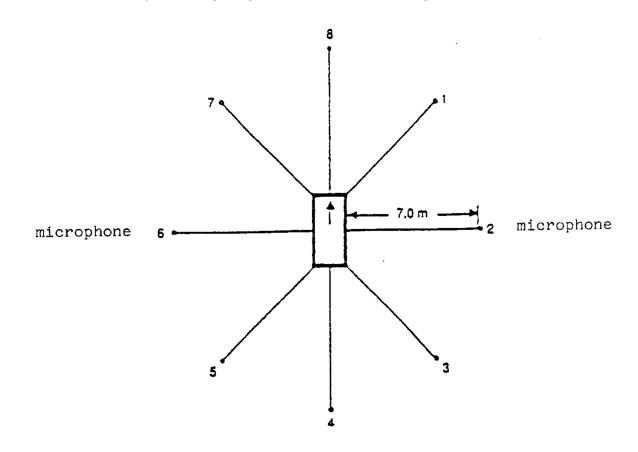
The measurement is performed at the stationary vehicle in accordance with Figure 1, using two microphone positions at a distance of 7 m from the contour of the vehicles and at 1,2 m above ground.
