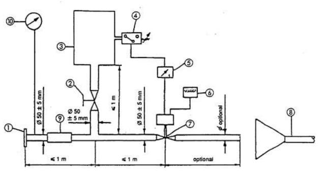
Figure 1 Test apparatus for conditioning by pulsation
