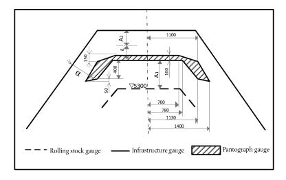
$Table\ D.1$  Distances between live parts of OCL and pantograph and earthed parts of rolling stock and fixed instalations for 1 520mm track gauge system
