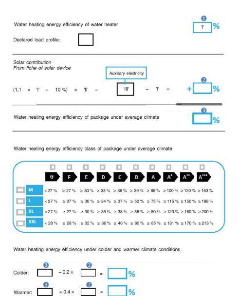
The energy efficiency of the package of products provided for in this fiche may not correspond to its actual energy efficiency once installed in a building, as this efficiency is influenced by further factors such as heat loss in the distribution system and the dimensioning of the products in relation to building size and characteristics.
