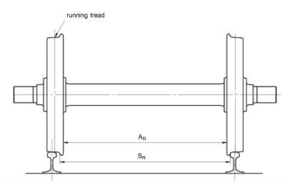
$\label{eq:able3} \textit{Limits of use of the geometric dimensions of wheelsets}$
