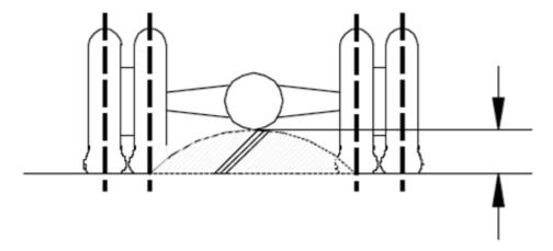
3.2.2. Where appropriate, the measurement of ground clearance shall be conducted on each of the several axles of a group of axles.
