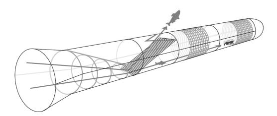
Schematic illustration of a size and species selective trawl. Entering fish is led towards the trawl floor and grid via a leading funnel. Larger fish is then led out of the trawl by the grid while smaller fish and Norway lobster pass through the grid and enter the codend. The full square mesh codend enhance escapement of small fish and undersized Norway lobster.
