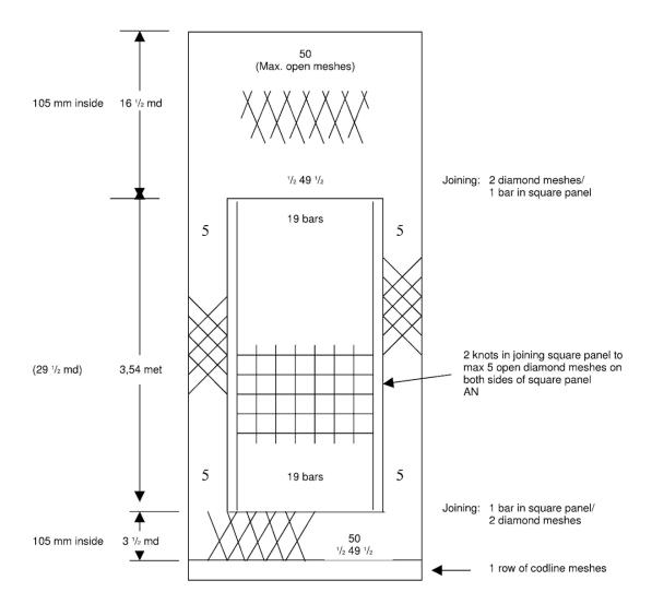
The construction of upper panel in case 20 % of diamond meshes in the upper panel are maintained and equally divided on both sides of the window
