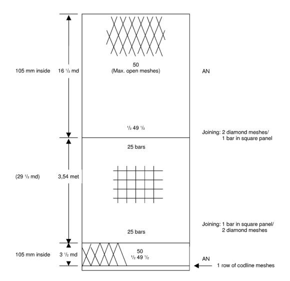
The construction of upper panel, size and position of the window panel in case when the escape panel runs from selvedge to selvedge
