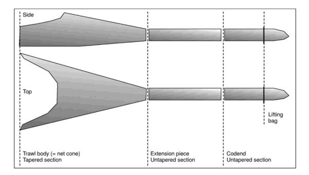
Trawl gear can be divided into three different sections according to shape and function.
