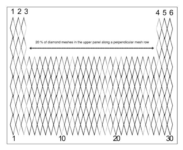
Twenty percent of diamond meshes in the upper panel along a perpendicular row running from one selvedge to another may be maintained. For example (as in figure 3) if the upper panel were 30 open meshes wide, 20 % of that would be 6 meshes. Then three open meshes are divided on both sides of the window panel. Consequently the width of the window panel then becomes 12 mesh bars (30 - 6 = 24 diamond meshes divided by two is 12 mesh bars).
