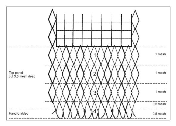
The distance of the window panel from the codline shall be 4 meshes. There are 3,5 diamond meshes in the upper panel and one 0,5 mesh deep hand-braided 'codline' row. Figure 3
