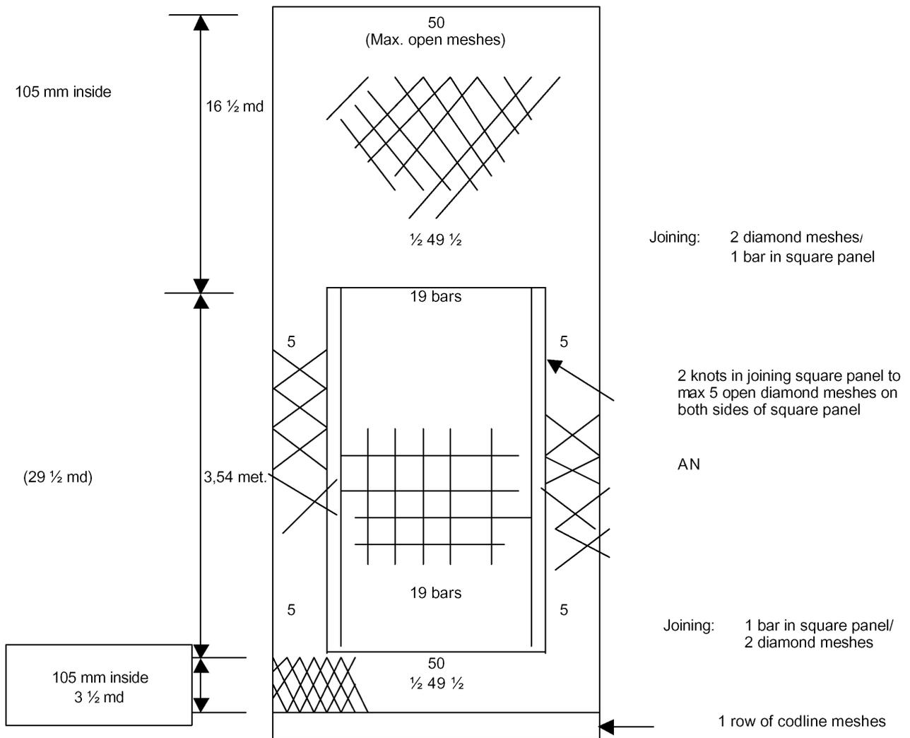
The construction of upper panel in case 20 % of diamond meshes in the upper panel are maintained and equally divided on both sides of the window.
