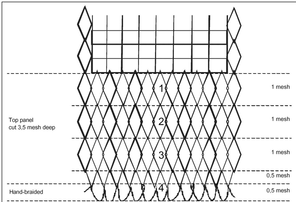
The distance of the window panel from the codline is 4 meshes. There are 3,5 diamond meshes in the upper panel and one 0,5 mesh deep hand-braided 'codline' row.
