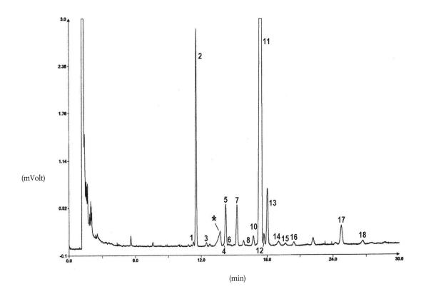
$Figure \ 2$  Gas chromatogram of the sterol and triterpene dialchols fraction of a refined olive oil (spiked with internal standard)
