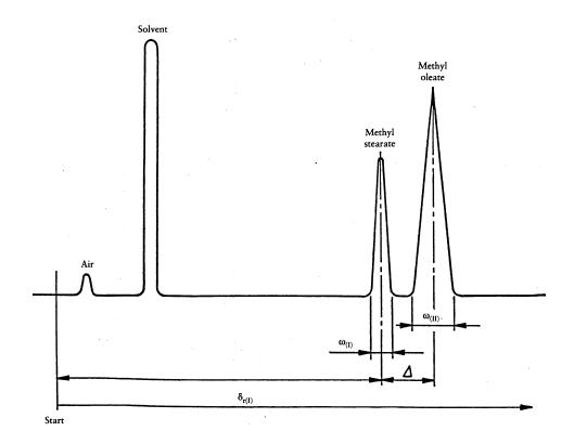
The operating conditions to be selected are those which will afford at least 2 000 theoretical plates per metre of column length for methyl stearate and a resolution of at least 1,25.
