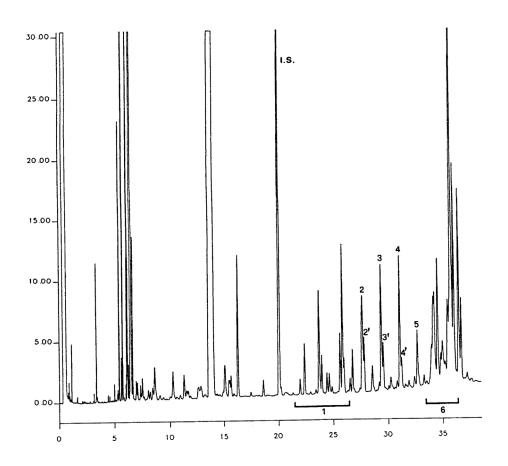
Peaks with a retention time from 5 to 8 min of the fatty acid methyl and ethyl esters
