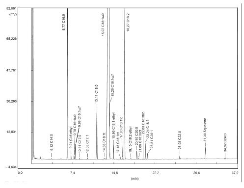
Figure 1: Gas chromatographic profile obtained by the cold methylation method from olive-pomace oil. The chromatographic peaks correspond to the methyl and ethyl esters except where otherwise indicated.
