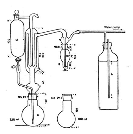
The gas feed tube to the bubbler B ends in a small sphere of 1 cm diameter with 20 0,2-mm diameter holes around its largest horizontal circumference. Alternatively, this tube may end in a frit glass plate which produces a large number of very small bubbles and thus ensures good contact between the liquid and gaseous phases.
