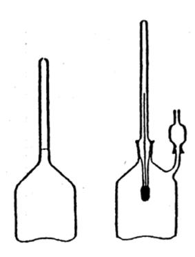
The pycnometer has a side tube 25 mm in length and 1 mm (maximum) in internal diameter, ending in a conical ground joint. This side tube may be capped by a 'reservoir stopper' consisting of a conical ground-glass joint tube and terminating in a drawn-out section. This stopper serves as an expansion chamber.
