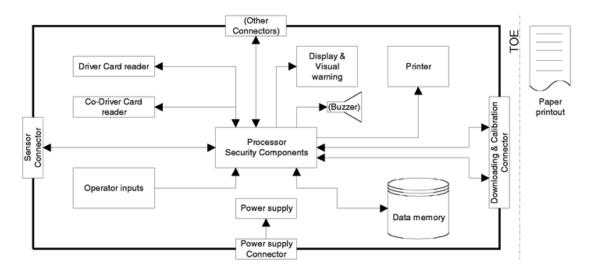
It must be noted that although the printer mechanism is part of the TOE, the paper document once produced is not.
