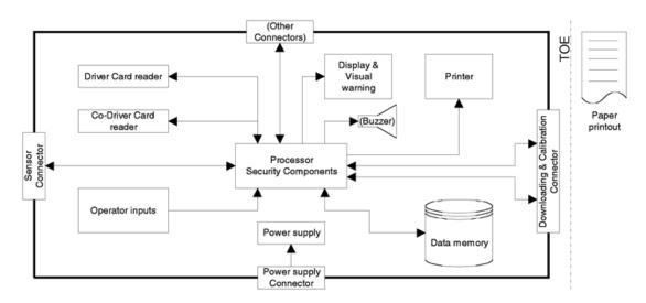
It must be noted that although the printer mechanism is part of the TOE, the paper document once produced is not.
