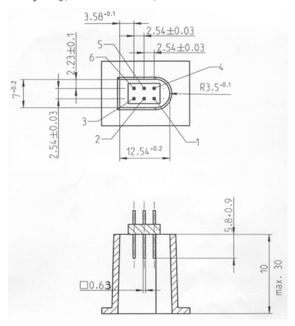
The following diagram shows a typical six pin mating plug:
