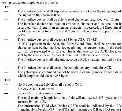
after the ATR and the card shall send back S-Block IFS. The recommended
