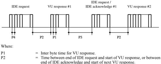
= Time between end of VU response and start of new IDE request, or between end of VU response and start of IDE acknowledge, or between end of IDE request and start of new IDE request if VU fails to respond.
