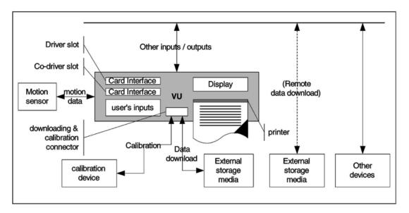
The VU general characteristics, functions and mode of operations are described in Chapter II of Annex I B.
