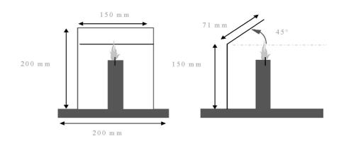
(e) The candle placed on the metal support shall be positioned midway between the two ends of the drum (Figure 6.3.2.3);
