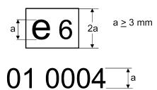
Legend: the above component type-approval was issued by Belgium under number 0004. 01 is a sequential number denoting the level of technical requirements to which this component fulfils. The sequential number is attributed in accordance with the relevant separate directive or regulation.
