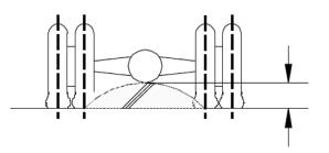
3.2.2. Where appropriate, the measurement of ground clearance shall be conducted on each of the several axles of a group of axles.
