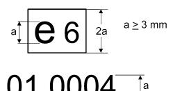
Legend: the above component type-approval was issued by Belgium under number 0004. 01 is a sequential number denoting the level of technical requirements to which this component fulfils. The sequential number is attributed in accordance with the relevant separate directive or regulation.
