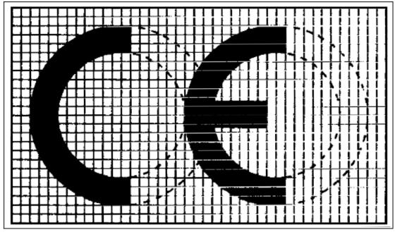
If the marking is reduced or enlarged the proportions given in the above graduated drawing must be respected.
