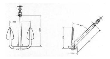
A tolerance of  $\pm 5$  % applies to the dimensions and mass given. However, the surface area of each fluke must be at least 0,15 m<sup>2</sup>.
