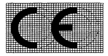
The CE marking must have a height of at least 5 mm. If the CE marking is reduced or enlarged the proportions given in the above graduated drawing must be respected.
