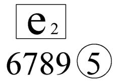
The above represented type-approval mark was issued by France  $[e_2]$  under number 6789 for the replacement catalytic converter not integrated in the exhaust system (catalytic converter and silencer not integrated in a sole element) (see Chapter 5).
