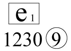
The above represented type-approval mark was issued by Germany  $[e_1]$  under number 1230 for the non-original silencer not integrating a catalytic converter (catalytic converter and silencer not integrated in a sole element or vehicle not equipped with a catalytic converter) (see Chapter 9).'
