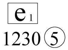
The above represented type-approval mark was issued by Germany  $[e_1]$  under number 1230 for the replacement catalytic converter not integrated in the exhaust system (catalytic converter and silencer not integrated in a sole element).
