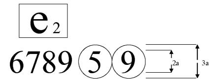
The above represented type-approval mark was issued by France [e<sub>2</sub>] under number 6789 for a non-original exhaust system consisting of a sole part integrating both the silencer and the catalytic converter.
