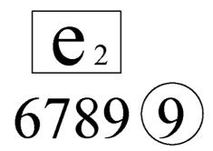
The above represented type-approval mark was issued by France  $[e_2]$  under number 6789 for a non-original silencer not integrating a catalytic converter (catalytic converter and silencer not integrated in a sole element or vehicle not equipped with a catalytic converter)
