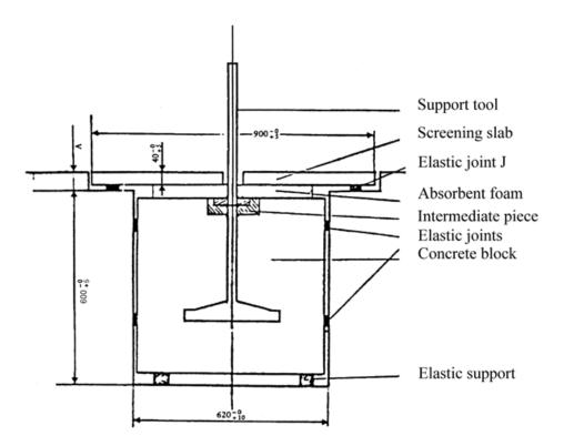
The value of A should be such that the screening slab resting on the elastic joint J is flush with the ground
