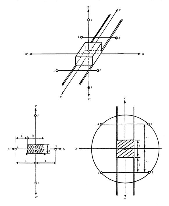
Arrangement of microphone positions where the lifting mechanism is located on the jib stay
