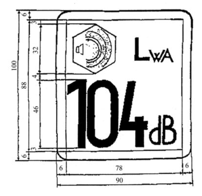
If the indication is reduced or enlarged according to the size of the equipment the proportions given in the above drawing must be respected. However, the vertical dimension of the indication should, if possible, not be less than 40 mm.
