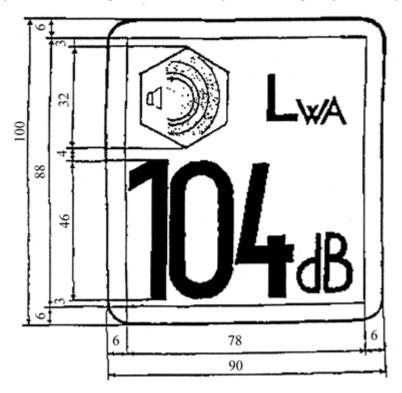
If the indication is reduced or enlarged according to the size of the equipment the proportions given in the above drawing must be respected. However, the vertical dimension of the indication should, if possible, not be less than 40 mm.
