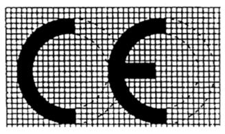
Iff the CE marking is reduced or enlarged according to the size of the equipment the proportions given in the above drawing must be respected. The various components of the CE marking must have substantially the same vertical dimension which may not be less than 5 mm.
