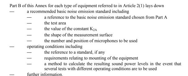
When testing specific types of equipment, the manufacturer or his authorised representative in the Community may in general choose one of the basic noise emission standards of Part A and apply the operating conditions of Part B for this specific type of equipment. In the event of a dispute, however, the recommended basic noise emission standard laid down in Part B has to be used together with the operating conditions of Part B.
