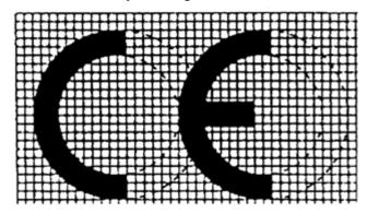
Iff the CE marking is reduced or enlarged according to the size of the equipment the proportions given in the above drawing must be respected. The various components of the CE marking must have substantially the same vertical dimension which may not be less than 5 mm.
