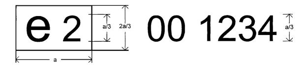
The above approval mark affixed to a component of a replacement catalytic converter shows that the type concerned has been approved in France (e 2), pursuant to this Directive. The first tow digits of the approval number (00) refer to the sequence number assigned to the most recent amendments made to Directive 70/220/EEC. The following four digits (1234) are those allocated by the approval authority to the replacement catalytic converter as the base approval number.'
