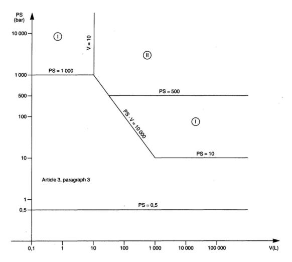
Exceptionally, all piping containing fluids at a temperature greater than 350 °C and falling within category II on the basis of Table 7 must be classified in category III.
