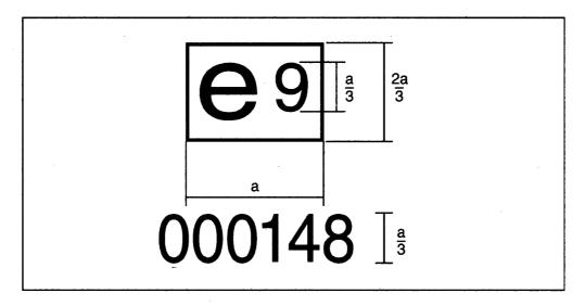
The windscreen washer system bearing the above EEC type-approval mark is a device which has been approved in Spain (e 9) under the base approval number 0148 on the basis of this Directive. The figures used are only indicative.'
