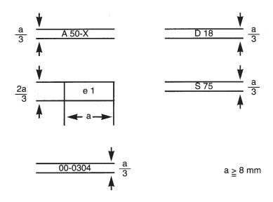
The coupling device with the EEC approval marking illustrated above is a non-standard coupling ball and towing brackets of Class A 50-X having a maximum permitted D value of 18 kN and a maximum permitted static vertical bearing load of 75 kg, for which EEC component type-approval was granted in the Federal Republic of Germany (e 1) under the number 0304. The first two digits 00 indicate that this component was approved according to the original form to this Directive.
