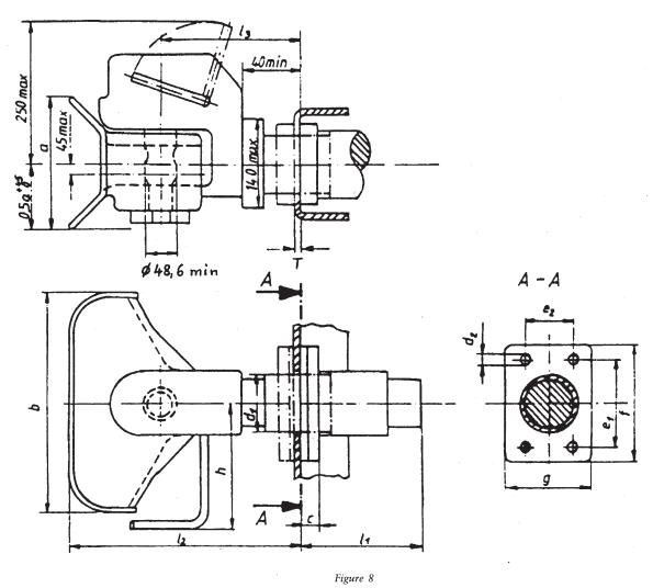
Dimensions of the standard drawbar coupling (mm) (see Table 3).
