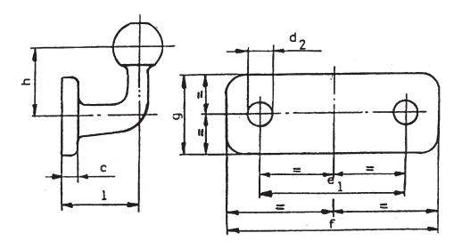
Figure 3 Dimensions of standard ball couplings and flange type towing brackets of Class A 50-1 (mm) (see Table 1)
