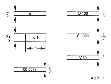
The coupling device with the EEC approval marking illustrated above is a drawbar for a centre-axle trailer of Class E with a maximum permitted D value of 109 kN, a maximum permitted static vertical bearing load of 1 000 kg and a maximum permitted V-value of 50 kN, for which EEC component type approval was granted in the Federal Republic of Germany (e 1) under the number 0013. The first two digits 00 indicate that this component was approved according to the original form of this Directive.
