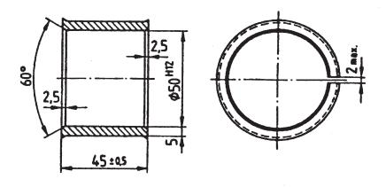
Figure 12 Slotted sleeve for D 50 drawbar eyes
