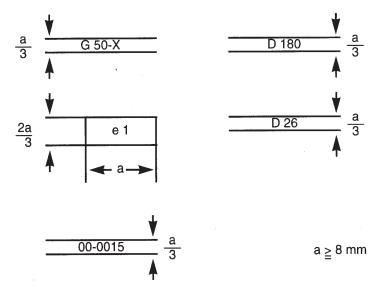
The coupling device with the EEC approval marking illustrated above is a non-standard fifth wheel coupling of Class G 50-X having a maximum permitted D value of 180 kN and a maximum permitted fifth wheel load of 26 tonnes, for which EEC component type-approval was granted in the Federal Republic of Germany (e 1) under the number 0015. The first two digits 00 indicate that this component was approved according to the original form of this Directive.
