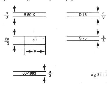
The coupling device with the EEC approval marking illustrated above is a non-standard coupling head of Class B 50-X having a D value of 18 kN and a maximum permitted static vertical bearing load of 75 kg, for which EEC component type-approval was granted in the Federal Republic of Germany (e 1) under the number 1993. The first two digits 00 indicate that this component was approved according to the original form of this Directive.
