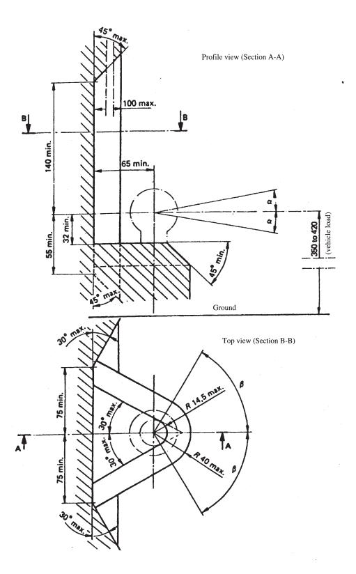
Figure 30 Clearance space for coupling balls
