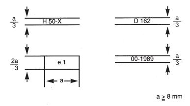
The coupling device with the EEC approval marking illustrated above is a non-standard fifth wheel coupling pin of Class H 50-X having a D value of 162 kN for which EEC component type-approval was granted in the Federal Republic of Germany (e 1) under the number 1989. The first two digits 00 indicate that this component was approved according to the original form of this Directive.
