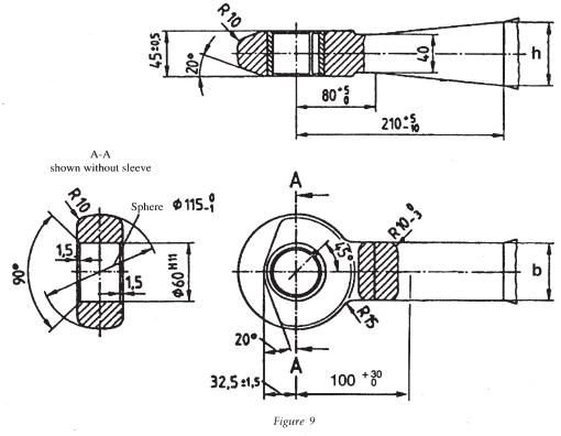
Dimensions of Classes D 50-A and D 50-X drawbar eyes (see Table 6)
