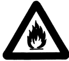
Flammable material or high temperature (1)
