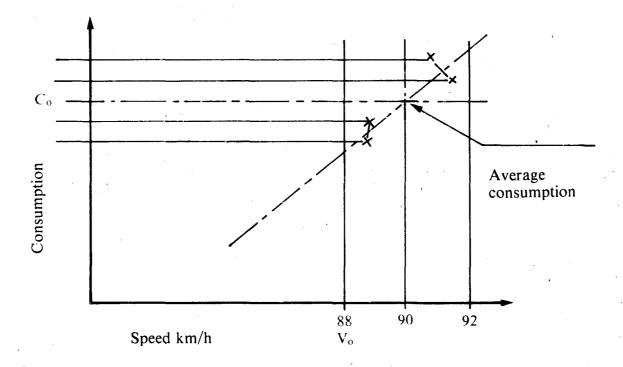
The four crosses correspond to the calculated values for each test run.  $C_o$  is the value calculated for the consumption at the reference speed  $V_o$  over the test distance.
