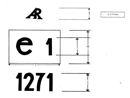
The device bearing the EEC component type-approval mark shown above is a reversing lamp EEC type-approved in Germany (e 1) under the number 1271.
